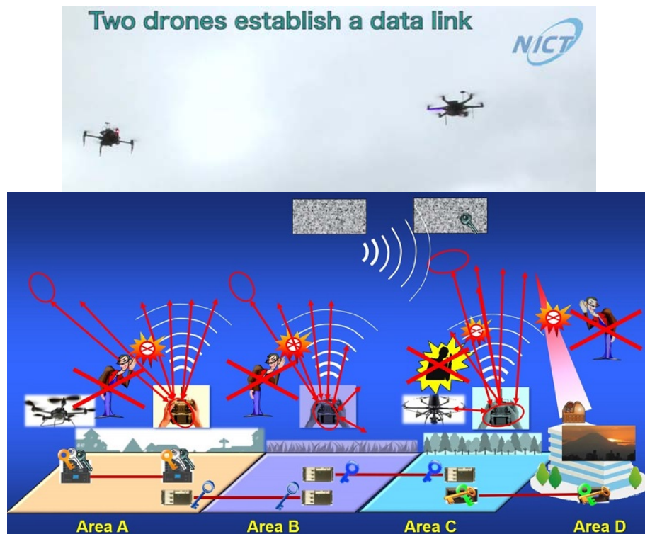
Figure 2.17. Demonstration of secure communications between drones (above), and how keys can be passed along as the drone travels over various regions (below)
