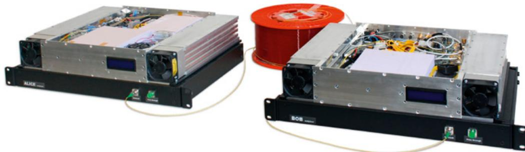
Quantum key distribution system: autonomous GHz-rate prototype, H. Zbinden, University of Geneva.
